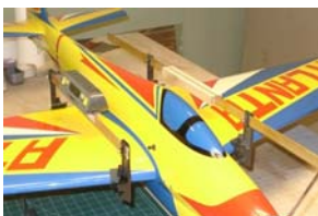
Balsa glued to bar to form flat mount area for level device.
