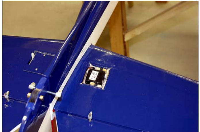
Tail wheel neatly enclosed in Dirty-Birdy rudder Micro servo in stab drives elevator
