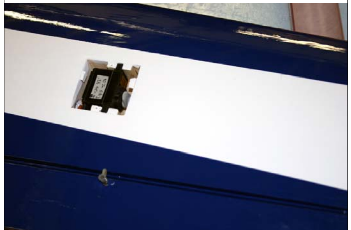
Aileron servo hatch-lid removed to reveal neat installation
